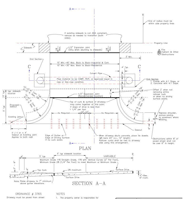
Driveway must be paved from street pavement to property line (or to existing sidewalk, with 3000# Portland Cement Concrete or type "B" Asphaltic Concrete. When using brick pavers, the section from the sawcut to the end of radius must be concrete or asphalt.
