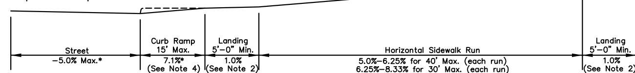
Sidewalk Ramp Profile (Not to Scale)
